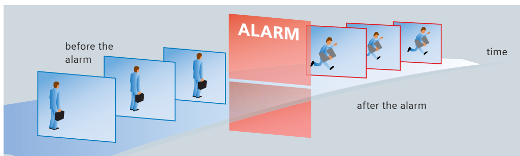
Eyetec stores images for an easy alarm evaluation.
